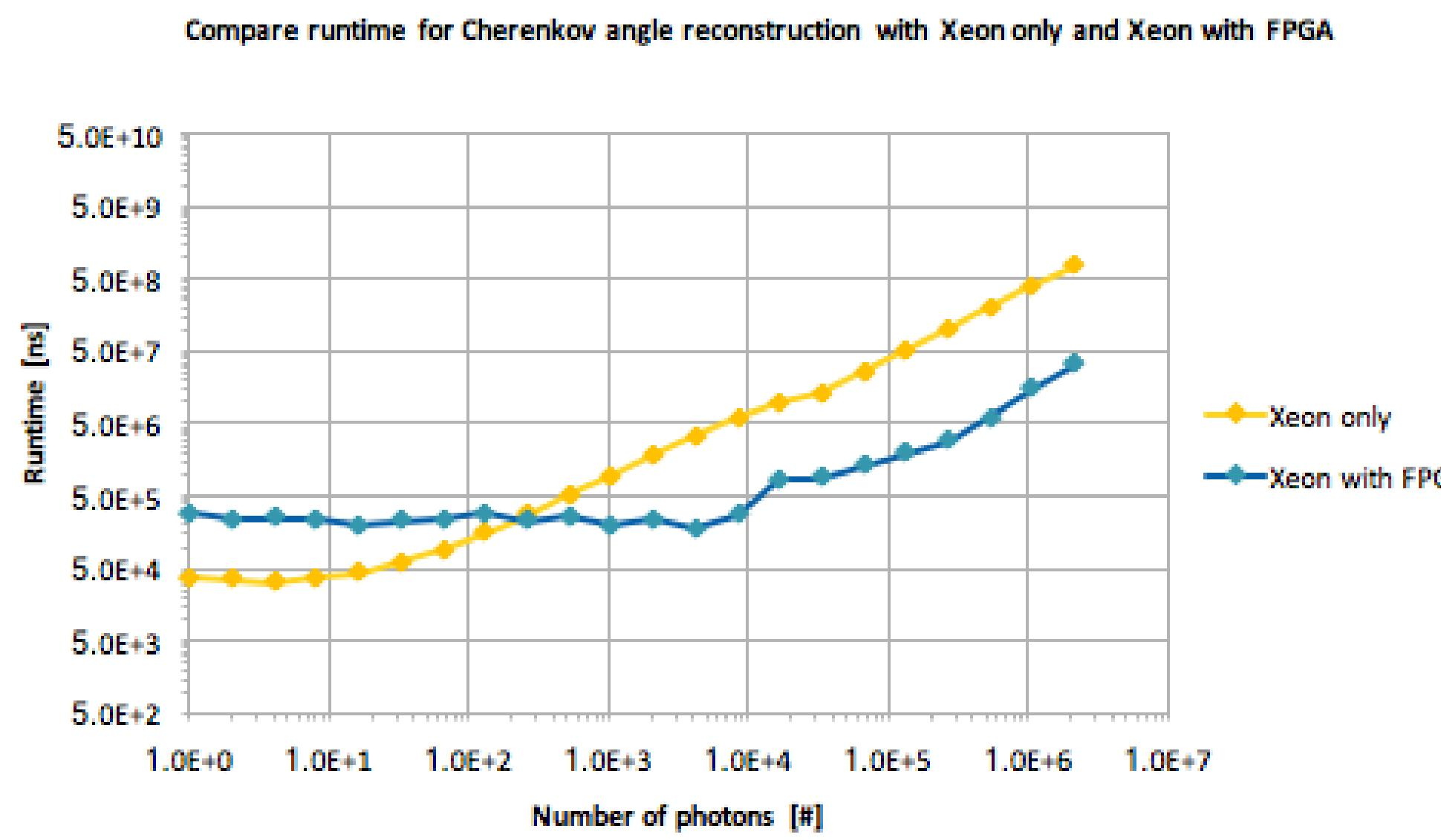
Acceleration of factor up to 35 with Xeon/FPGA
